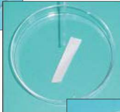
STEP 2: Prepare inoculum and touch filter paper with loop
